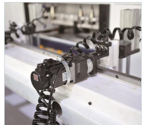
Automatic positioning for servo-driven clamps
